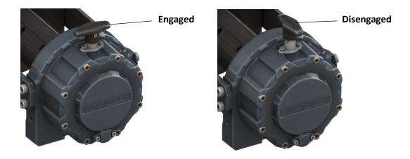
DO NOT ATTEMPT to pull a load until the drum is properly engaged.
